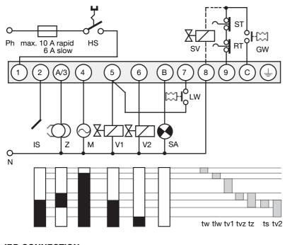
Gas pressure switch GW ST Limit thermostat Control thermostat RT IS Ionization probe Ignition Ζ Μ Burner motor Solenoid valve 1st stage V1 V2 Solenoid valve 2nd stage LW Air pressure monitor External fault indication SA SV Safety valve Waiting time at start-up tw
