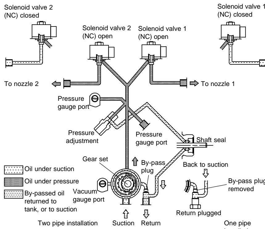
design ensures extremely fast response and the switching can be selected according to the burner operating sequence and is independent of motor speed.
